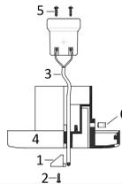
2. Put mains cable (3) through the opening in luminaire's base (4) and connect it to lampholder according to polarity.
