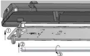
8. Replace the diffuser on luminaire's body and fix it with the snap locks.
