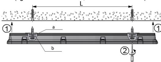
2.2. Suspended installation. Drill mounting holes in the luminaire's body, L – distance between holes: (on fig. a – M6 steel washer; b - rubber washer; c- M6 nut)
