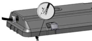
4. Connect mains cable to terminals on mounting panel according to polarity shown.
