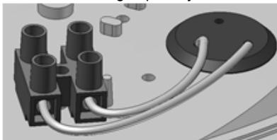
6. Fix the reflector on the luminaire's body. Install lamp.
