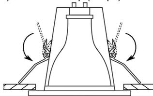
10. Replace diffuser (frame) by clicking it into luminaire's body with springs (external glass - by screws or springs).
