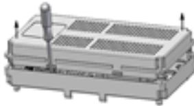
3.1.3. Put mains cable through hole in remote module, through strain relief next and connect to terminal block according to polarity shown.
