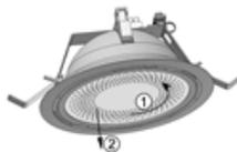
2. Remove reflector (for models with mounting brackets fixe).
