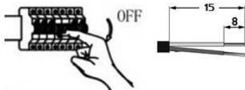
4. Connect mains cable to control gear's terminals according to scheme and polarity: "L" - phase conductor, "N" - negative conductor, the protective cover should be previously removed. Replace and secure control gear's protective cover.
