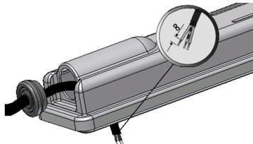
5. Connect mains cable to terminals on mounting panel according to polarity shown.
