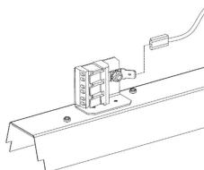
10. Connect the power and control wires to the terminal block in accordance with the specified polarity.
