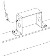
9. For grounding of luminaire body connect ground wire of each body to ground terminal in terminal block.
