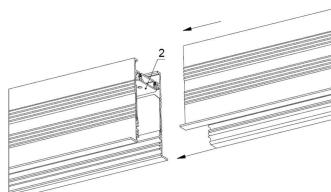
6.2. Move joining bracket on to next body and lock its position with 2 M4x8 screws. Tightening torque should not exceed 0,4 Nm.
