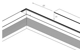
13. Diffuser joining in angle versions should be done at 90 degrees angle as shown on figure. In this case legs of longer diffuser should be cut on 3-5 mm with file or cut pliers.
