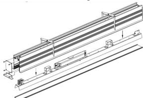
4. To prepare the installation cutout and to strip the power wire in accordance with the illustrations.
