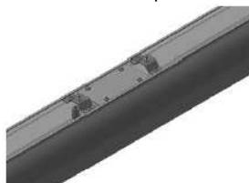
6. Fasten luminaires between each other with link (bringing luminaire right up to previous one) inside body.
