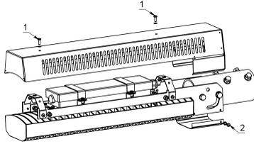
2. Set mounting bracket in desired position, adjust luminaire position by setting the angle needed (5 degrees step), tighten the screws (tightening torque 9 Nm).
