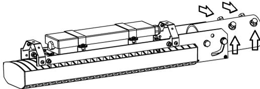
4. Replace cover back and tighten the screws (pos. 1).
