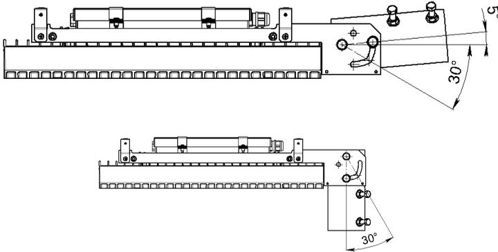
3. Mount luminaire on support with 4 bolts M8x35 (tightening torque 9 Nm).
