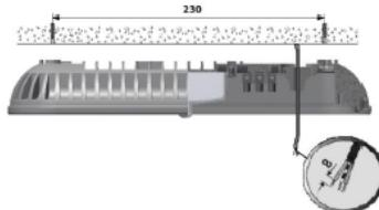
5. Attach the body to ceiling surface with X5 fasteners kit (not included), having put rubber washers (included) on screws beforehand. For luminaires with motion sensor mounting height is 1.5-3.5 m.
