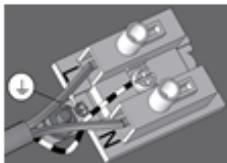
6. Connection polarity of mains conductors «+» and «-» to terminals L и N doesn't specified.
