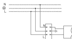
2. Mains connection scheme for luminaire with 1-10V dimmable driver.
